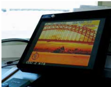
The radar shadow and visibility issues cast by the Sydney Harbour Bridge is not an issue with thermal imaging technology.
