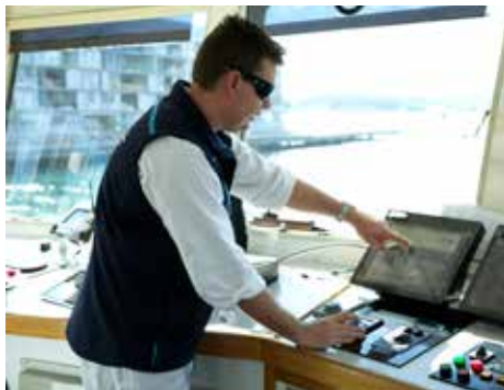
The ergonomic M-Series joystick control unit provides ready access to all critical system functions and smooth, effortless control, even in rough seas.
