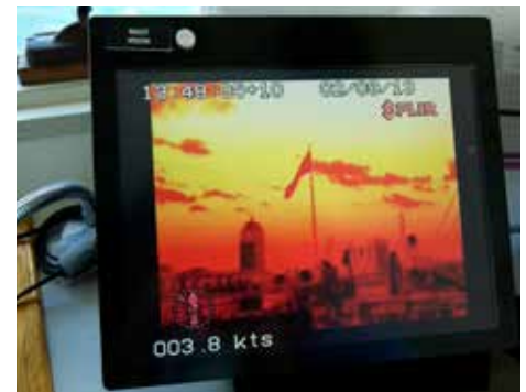
Different display settings let the operator choose between two black and white or three color display schemes that are easy on the eyes and help operators see better.
