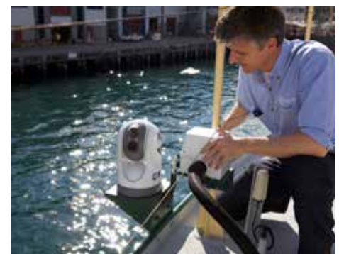
The compactness of the M-Series thermal imaging cameras allowed them to be accommodated within real estate constraints of what was already fitted to each vessel.
