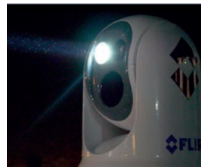
Integrated high intensity search lamp aids in target identification and crew coordination.
